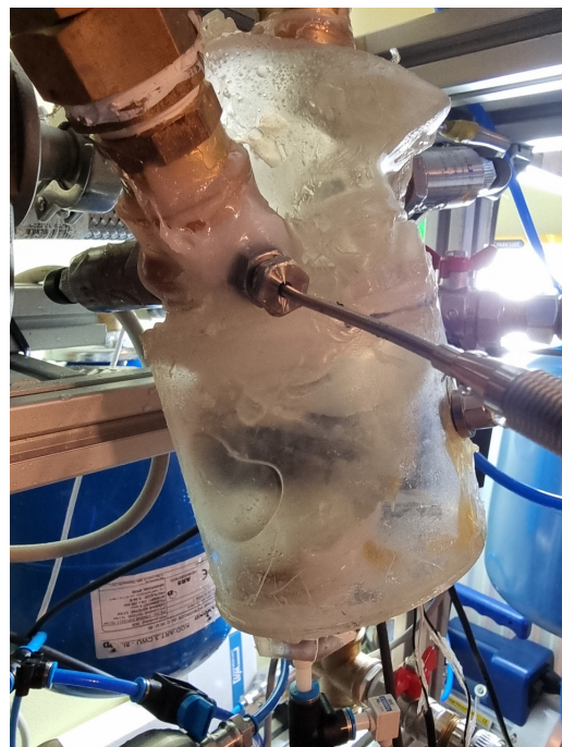
Figure 5. Flexible left heart model in a transparent cylinder—experimental stand.
