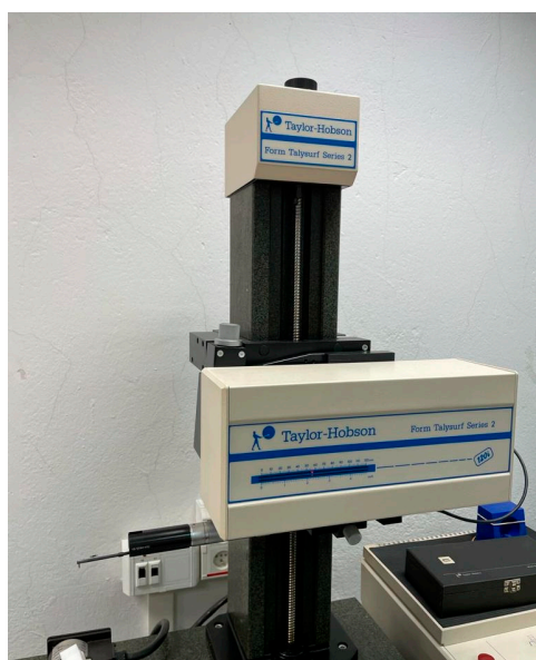
Figure 3. Taylor Hobson Talysurf 2 contact roughness meter.
