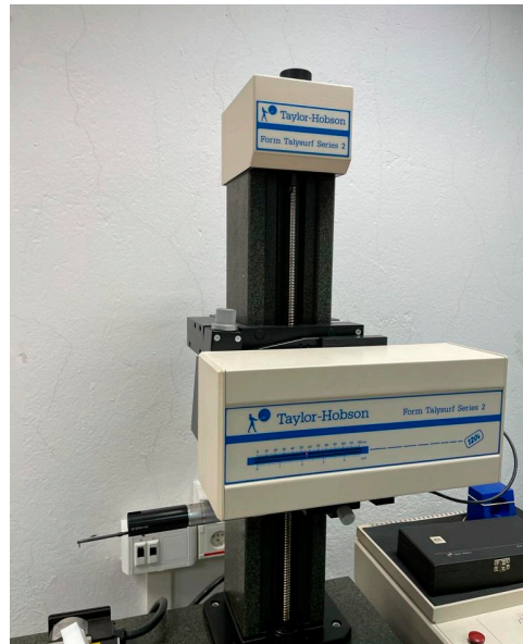
Figure 3. Taylor Hobson Talysurf 2 contact roughness meter.
