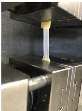
FIG. 6. Latex threads specimen in the Zwick Roell Z020 machine grips.
