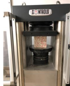
Fig.5: The compressive strength test.
