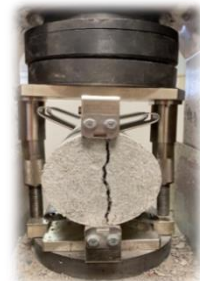
Fig.6: The splitting test.
