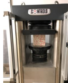
Fig.5: The compressive strength test.
