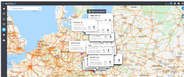
Fig. 4. The effect of sensors grouping in order to get a summary view of the railway transport fleet, managed by a particular user
