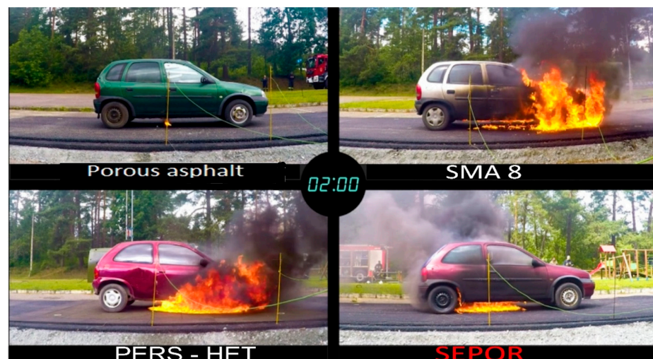
Figure 35. Fire development 120 s after ignition.
