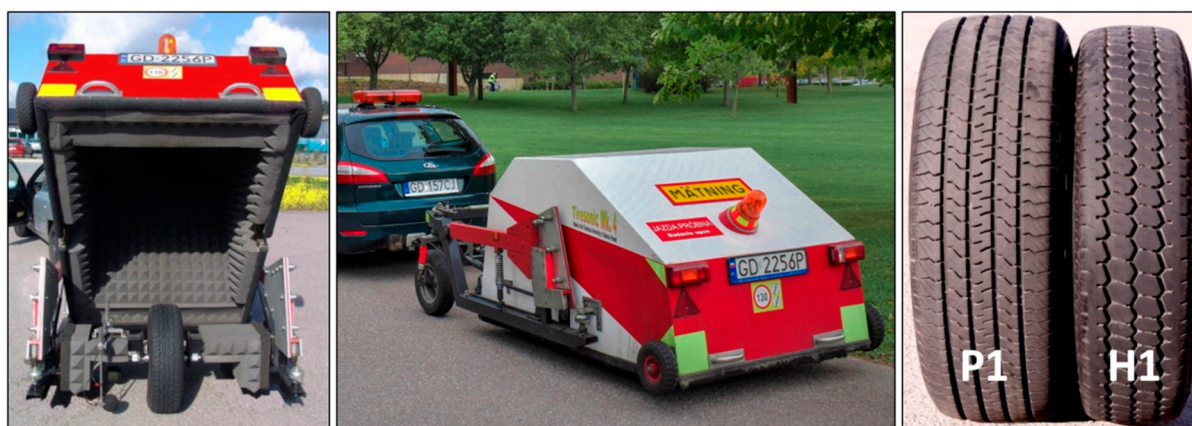
Figure 21. CPX test trailer Tiresonic Mk4 and the two ISO reference test tyres used: P1 and H1.
