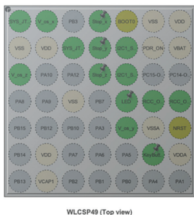
Fig. 13. Configuration of peripherals in STM32F411
