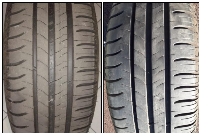
Fig. 8. Test tyres used in 2017 by the French CPX car: Michelin Energy Saver+ (left) and Michelin Energy Saver (right)
