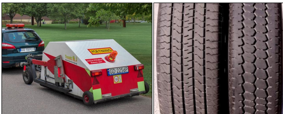
Fig. 2. CPX measuring system no. 2 – Polish test trailer Tiresonic Mk4 (left) and the test tyres used – two ISO reference tyres P1 and H1 (right)
