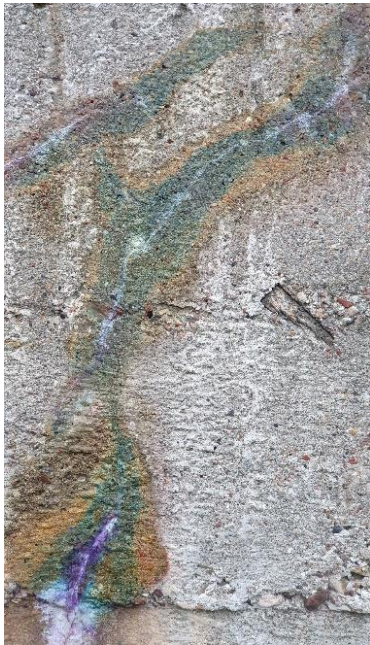
Photo 5: Discoloration of concrete after the Rainbow Test on the concrete surface, in the place of a crack on the wall of the right annex - test site after the test: a) view, b), c) close-up: green-violet coloration indicates advanced carbonation of concrete and its reduced ability to protect the reinforcement, the orange color indicates advanced carbonation of the exposed concrete surfaces, washing out of calcium carbonates is visible in the area of cracked concrete fragments
