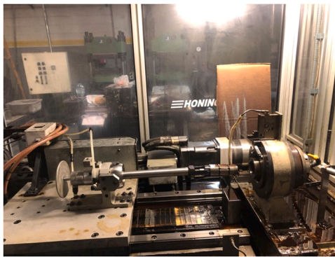
Fig. 1. Honing test machine from Honingtec S.A.
