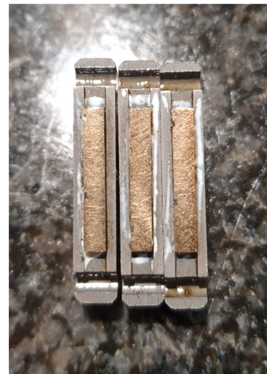
Fig. 3. cBN abrasive stones with metallic bond.
