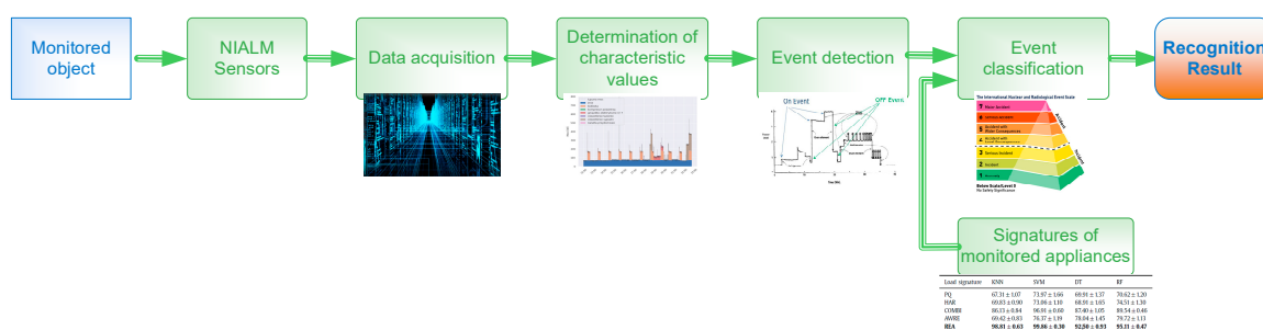
Figure 2. An example architecture of the NILM system.
