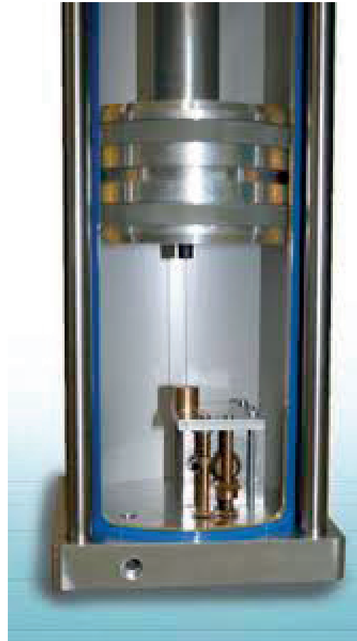
Fig. 1. Photo of the actuator with a magnetostrictive sensor located at the bottom of the cylinder
