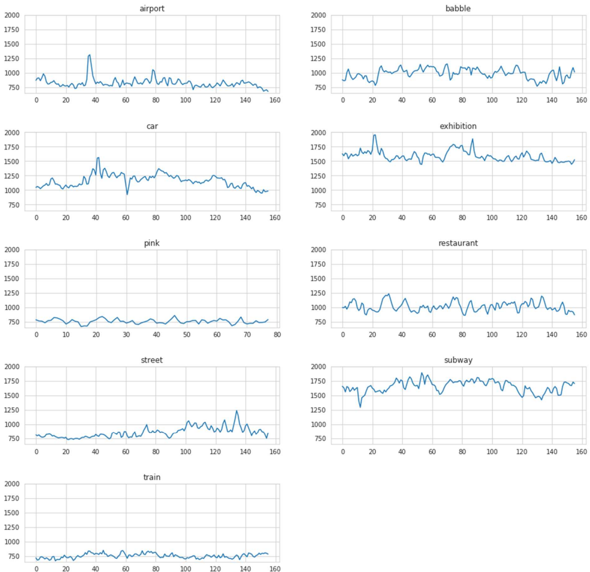
Figure 4.36 Spectral centroid of noise recordings
