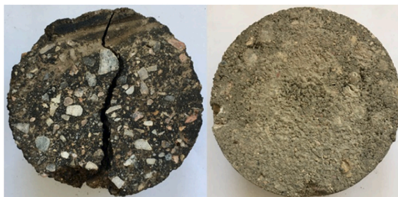
Fig. 3. Specimens after failure in the stiffness modulus test.
