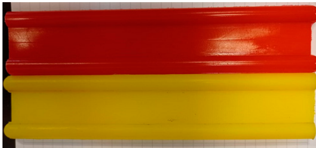
Figure 1. PS (pure shear) specimen geometry (width W = 140 mm, thickness t = 2 mm, effective height h = 15 mm) for relaxation test.
