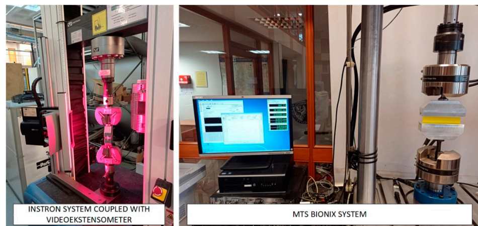
Figure 3. Experimental set-up for pure shear (PS) testing using Instron and MTS test system.
