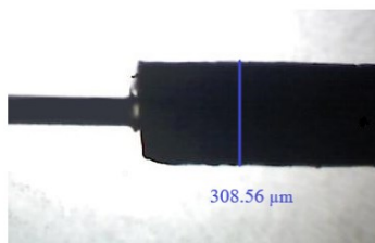
Figure 1. Fabricated SPME fibre with its diameter at 50 times magnification.
