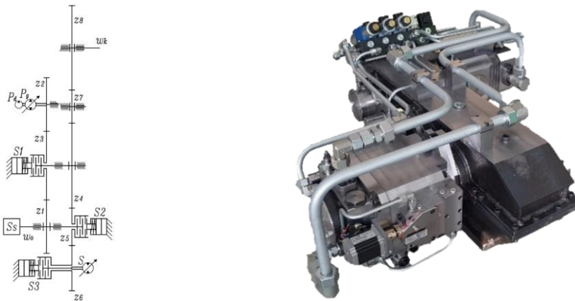
Fig. 1. Kinematic scheme and photo of hydromechanical gearbox
