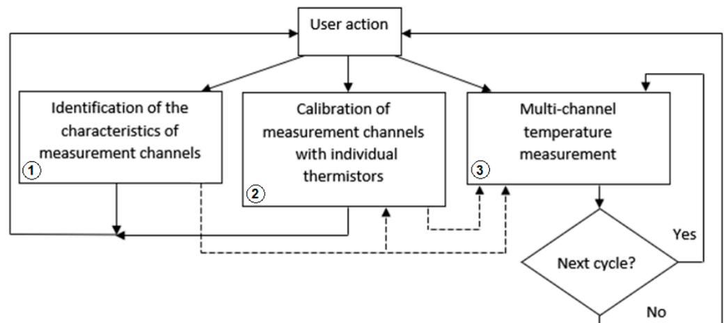
Figure 4. Block diagram of calibration and measurement procedures.
