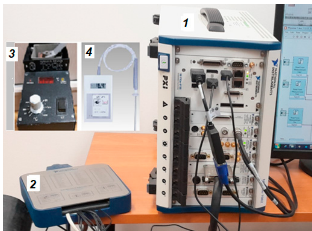
Figure 1. Developed multi-channel instrument and components for testing and calibration: 1—NI PXI measurement platform with NI DAQ card, 2—NI terminal block, 3—temperature calibrator, 4—digital thermometer.
