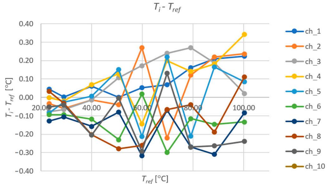
**Figure 6.** The course of differences between the temperatures determined in ten channels and the reference temperatures in relation to the reference temperatures ( $T_{ref}$ ).
