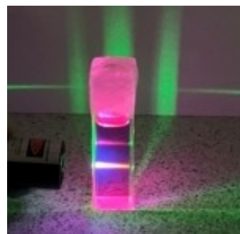
Figure 6. Digital photograph of up-converted emission from 5\text{ }\mu\text{M} B2PI and 50\text{ }\mu\text{M} perylene in deaerated dioxane at 532\text{ nm} (power density 1.27\text{ W cm}^{-2} ) excitation.
