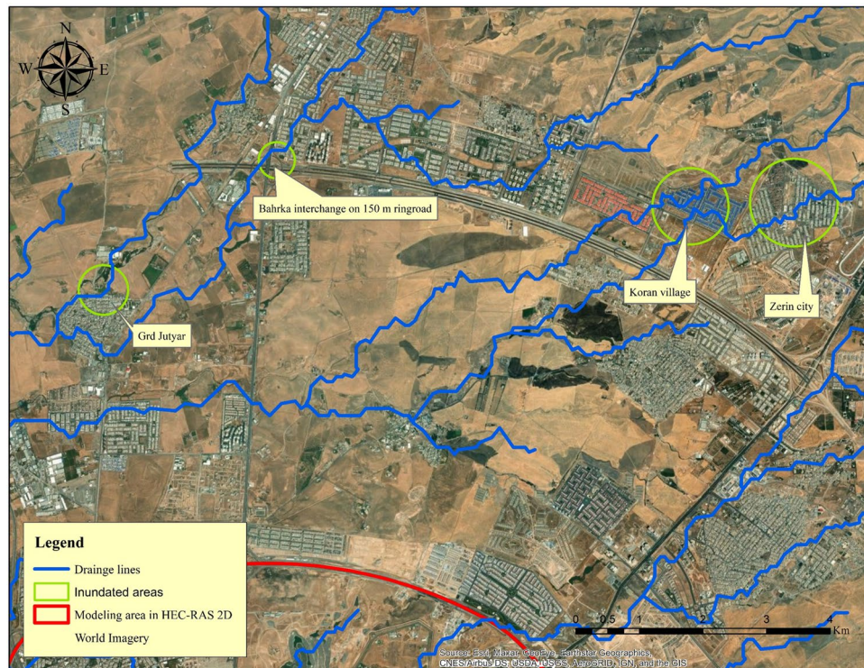
Figure 13. Some inundated areas in Erbil during the storm event of October 30 and December 17, 2021. Base imagery sources: Esri, DigitalGlobe, GeoEye, i-cubed, USDA FSA, USGS, AEX, Getmapping, Aerogrid, IGN, IGP, swisstopo, and the GIS User Community. This map is processed and generated in ArcGIS 10.7 software (© ESRI, URL: https://www.esri.com/en-us/arcgis/products/index ).
