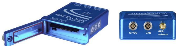
Fig. 4. GPS receiver used to determine the position of the vehicle and its altitude. GPS, Global Positioning System
