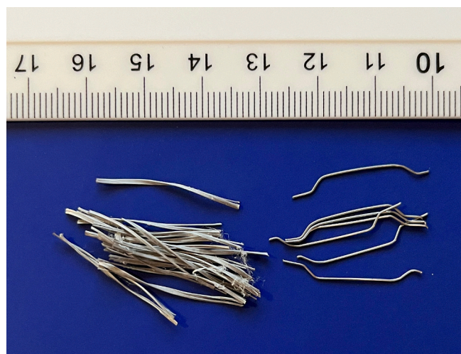
Fig. 1. Photograph of polyolefin fibres (left) and steel fibres (right).
