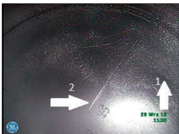
c) Piston crown – visible traces of carbon deposits (1) and scratches on the surface (2)
