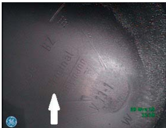
a) Piston head with visible identification number
