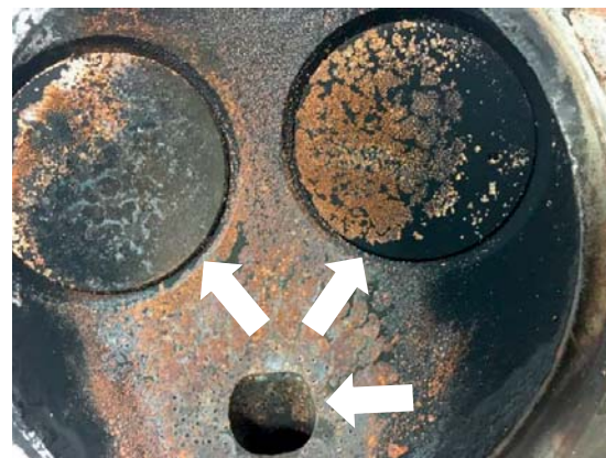
Bottom plate of the cylinder head – closed cylinder valves, a passage connecting the cylinder working space with the combustion pre-chamber, no traces of working medium leakage through the valve faces
