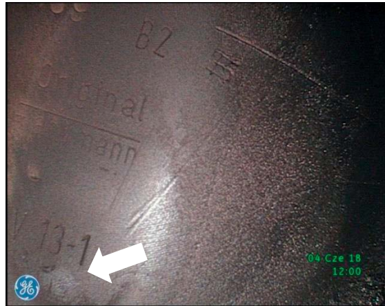
Fig. 9. Endoscopic image of the piston crown of the Farymann Diesel D10 research engine after testing RMG380 type marine fuel – surface clean, free of defects and contamination, identification numbers visible again
