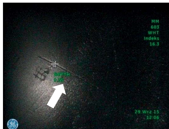
f) Measurement of the scratch depth on the piston crown made by the 'Shadow' method – 0.35 mm, with an accuracy index of 16.3, corresponding to an absolute error of 0.1 mm
