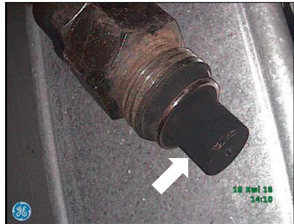
h) Fuel injector removed from the cylinder head – thick layer of soot on the spray tip
