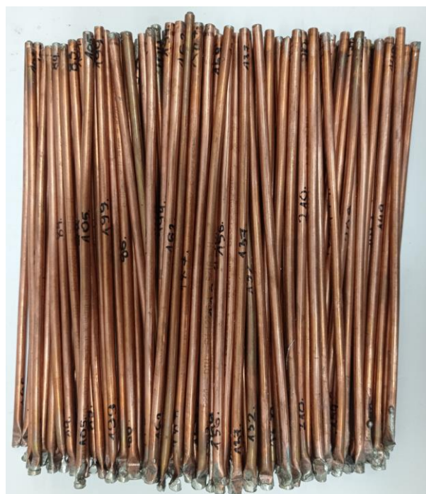
Figure 19. View of all 210 manufactured heat pipes.
