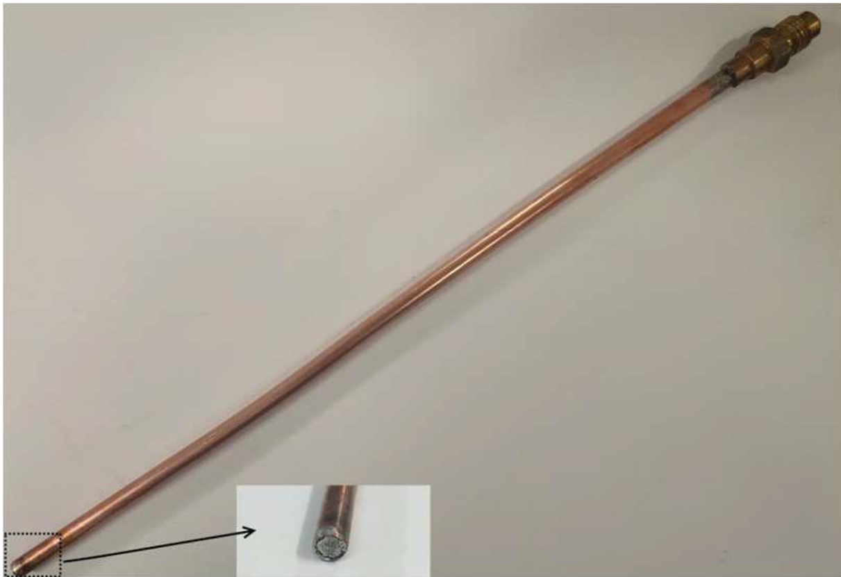
Figure 4. Photo of a heat pipe with a mesh inserted, soldered with a Shrader valve and a plug.
