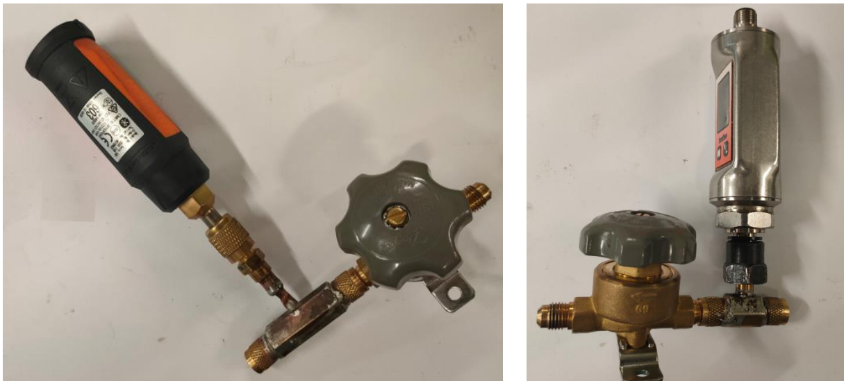
Figure 5. View of the fittings equipped TESTO 549i pressure sensor and a Danfoss BML 6 globe valve (left) and TRAFAG DCS6.0AR pressure transducer and a Danfoss BML 6 globe valves (right).
