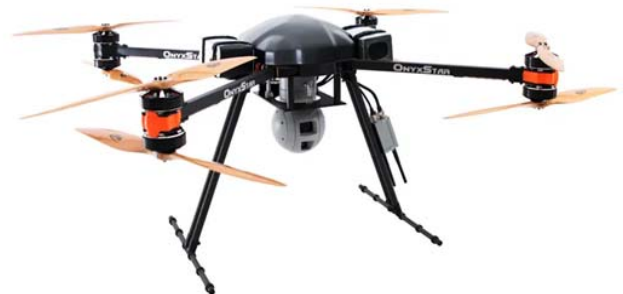
Figure 9. FOX-C8 XT UAV manufactured by OnyxStar [56].
