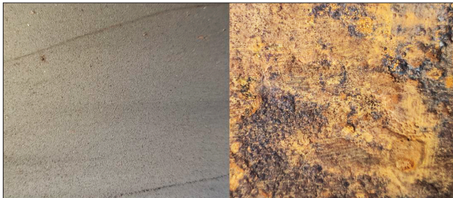
Fig. 3. Plate surface close-up. Left: intact plate. Right: c24 plate corroded and cleaned from corrosion products
