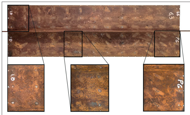
Fig. 4. Sample c12 (12% DoD): stiffener side view with close-ups of surface.
