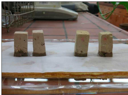
Figure 10. Hydraulic conductivity test.
