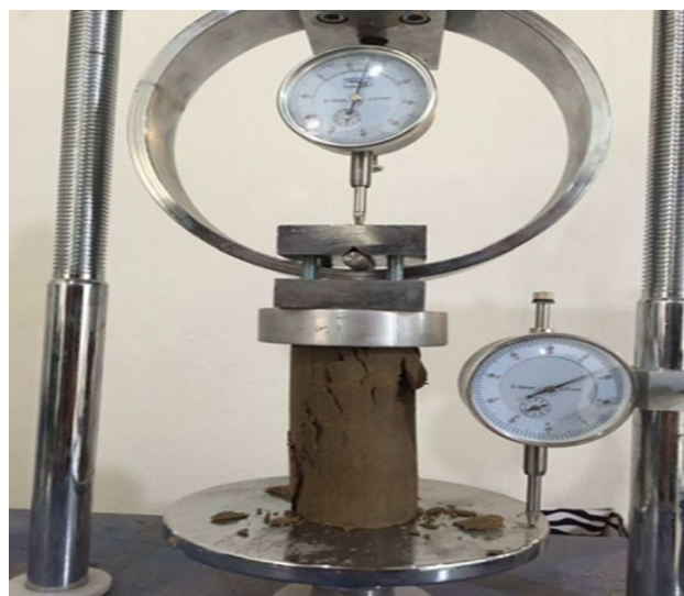
Figure 4. Specimen image after the UCS test.
