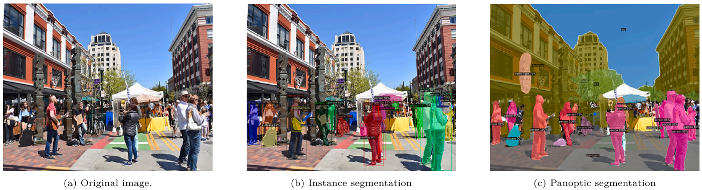
Fig. 1. Example of image segmentation using Mask RCNN (Region-Based Convolutional Neural Network) from Detectron 2 library (Wu et al., 2019) framework on image created by Tamaoekonomico, CC BY-SA 4.0, via Wikimedia Commons. It should be noted that the used image does not belong to the COCO dataset on which the Detectron 2 network was trained.
