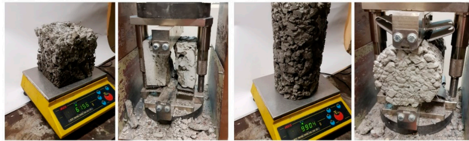
Figure 4. Cubic and cylindrical samples during Tensile splitting strength tests.
