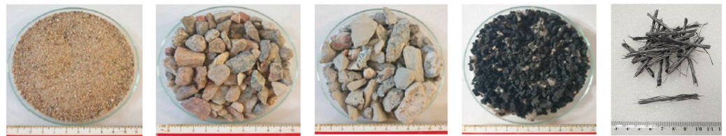
Figure 1. Fine Aggregate (0/2 mm, FA), Natural Coarse Aggregate (8/16 mm, NCA), Recycled Concrete Aggregate (8/31.5 mm, RCA), Rubber Waste Aggregate (2/5 mm, RWA), Polymer Fibers (54 mm length, PF).
