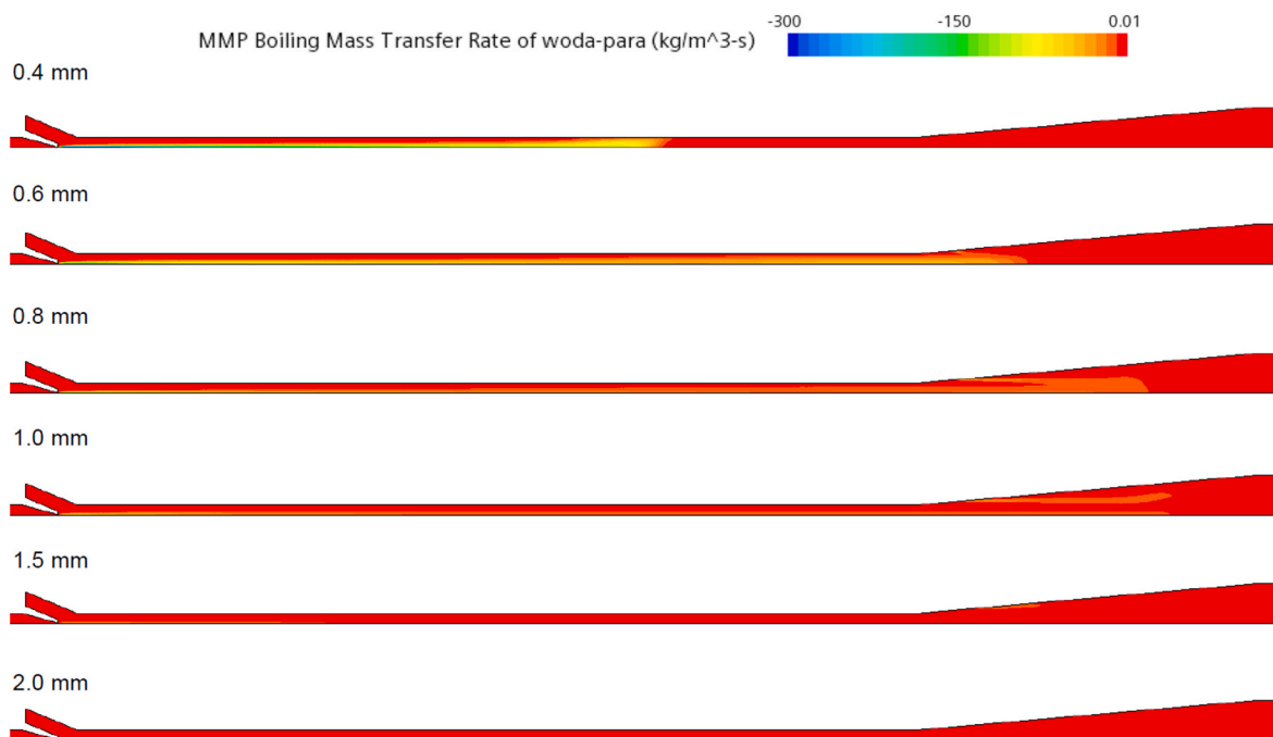
Fig. 15. Boiling/Condensation mass transfer rate field for various droplet size.
