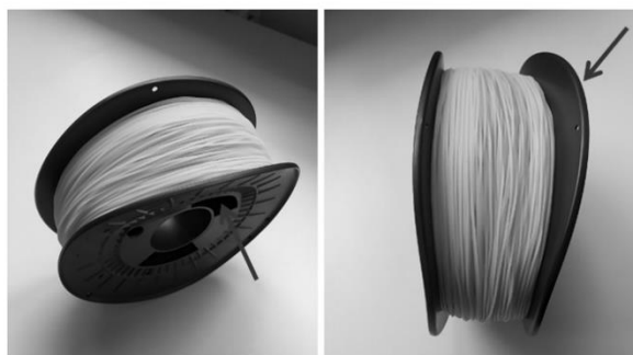
Figure S1. Damaged spool of TPU filament due to excessively high extrudate stresses generated during forming and winding process.
