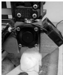
Figure S2 Scheme of the initial FDM 3D printing of heart by using F-TPU.
