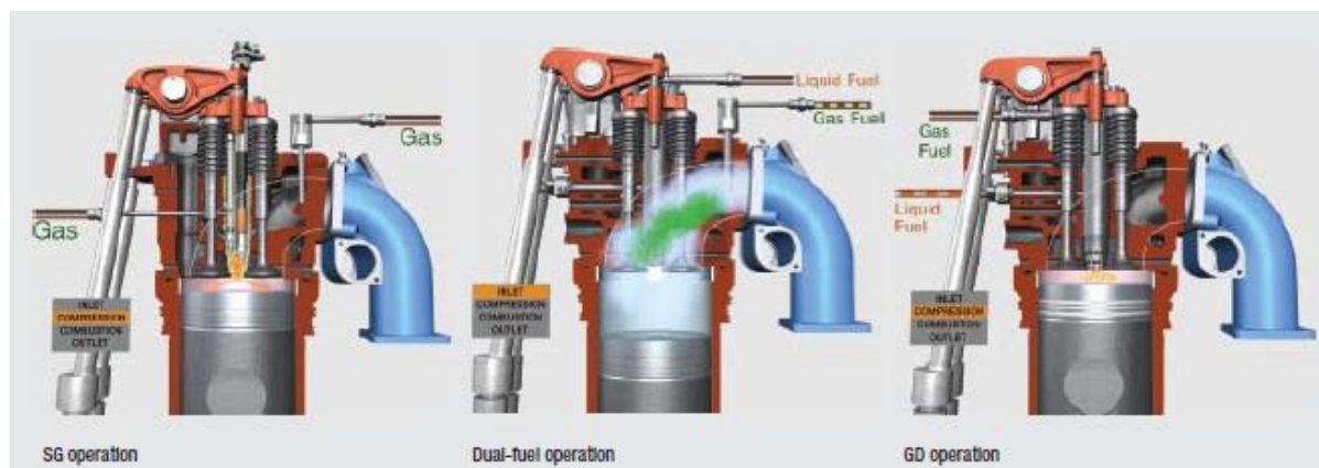
Fig. 12. Tree systems of 4 stroke engine operations: SI, dual fuel, diesel [11]
