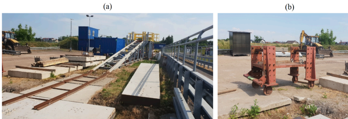
Fig. 9. View of (a) the crash test bench and (b) the test vehicle.
