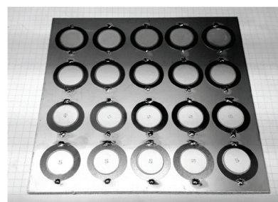
Fig. 4. PZT converter, consisting of 20 PZT/brass disk transducers fixed to a common copper surface.
