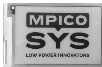
Fig. 7. The 2.71" black and white e-paper display used in the present study, with an example of graphical content.
