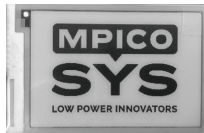
Fig. 7. The 2.71" black and white e-paper display used in the present study, with an example of graphical content.
