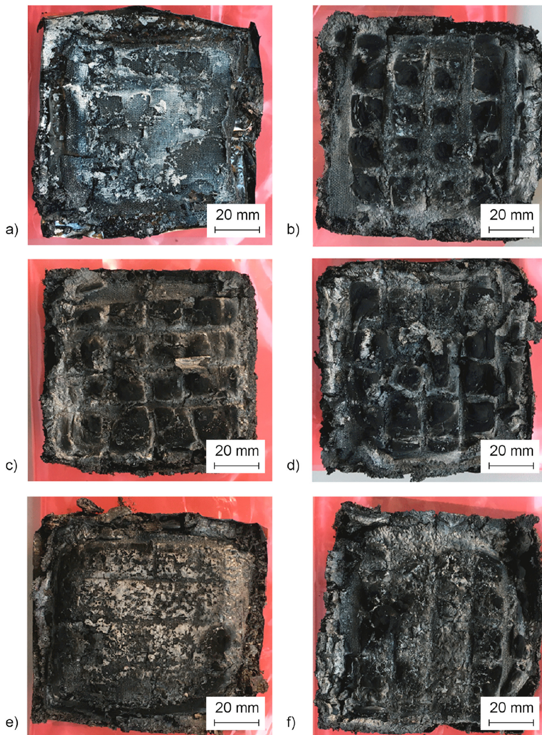
Fig. 9. Photographs of samples after cone calorimetry tests a) EP/FF, b) EP/FF/APP, c) EP/FF/APP/1VMT, d) EP/FF/APP/2VMT, e) EP/FF/APP/5VMT, f) EP/FF/APP/10VMT.
