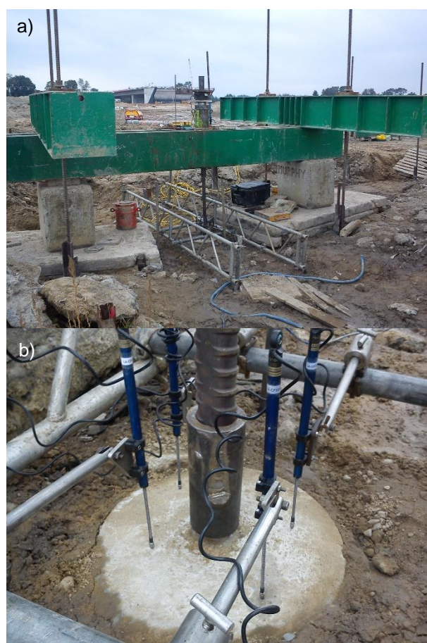
Photograph 5.1 a) The stand in pull-out test b) The measurement system
