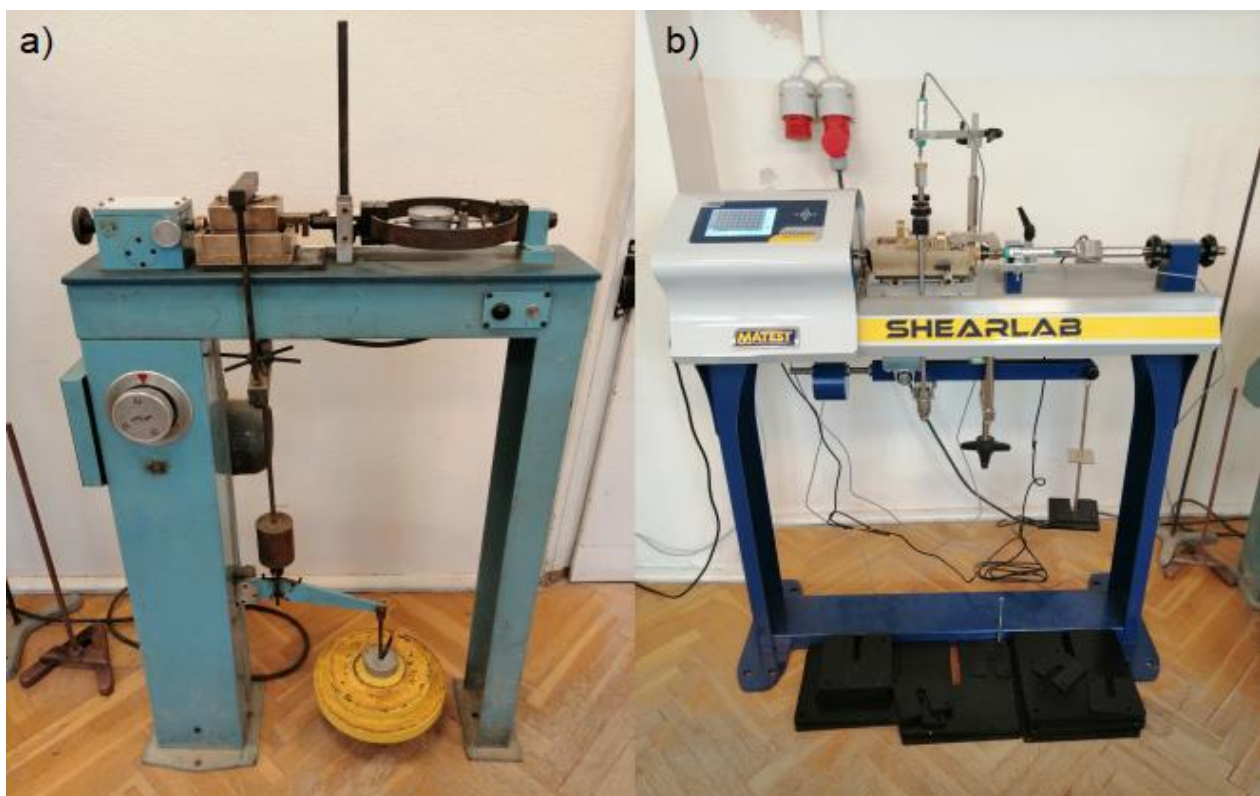
Photograph 6.2..a) analog direct shear apparatus b) digital direct shear apparatus
