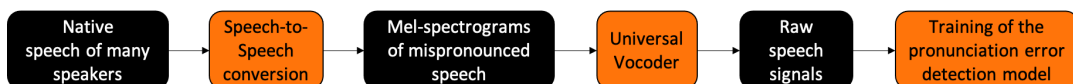
FIGURE 1.6: A single universal vocoder serving the generation of mispronounced speech across multiple speakers.
