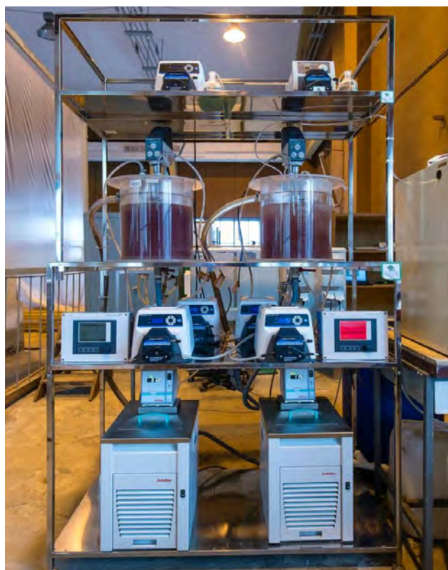
Figure 5- Experimental setup (SBR) at the laboratory of the university
