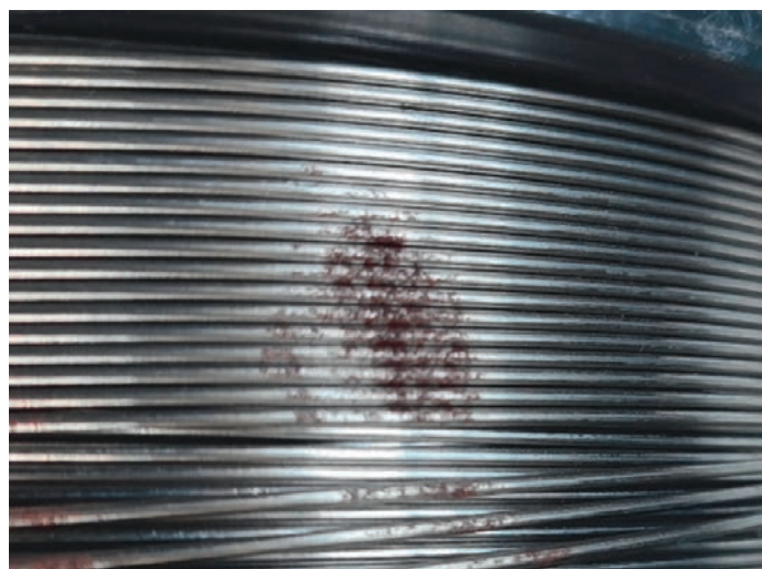
Fig. 2. Corrosion products on the wire surface in the area touched with the finger
