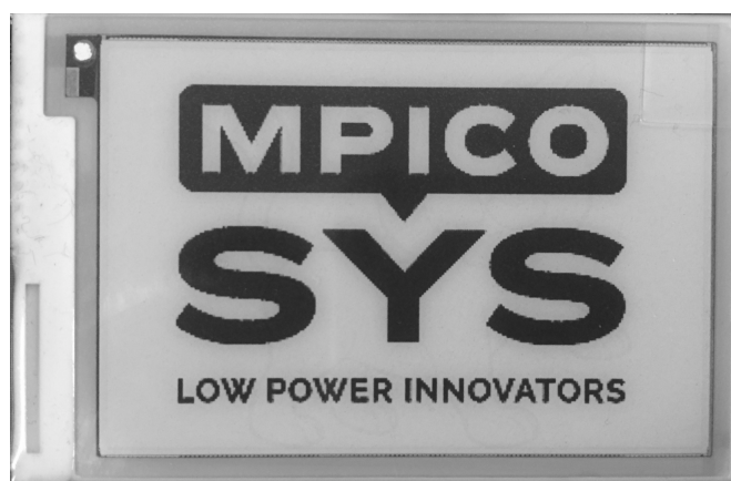
Figure 1. The 2.71" monochrome e-paper display considered in the use case scenario—the actuator of the IoT node powered with the use of the designed ES. [39]
