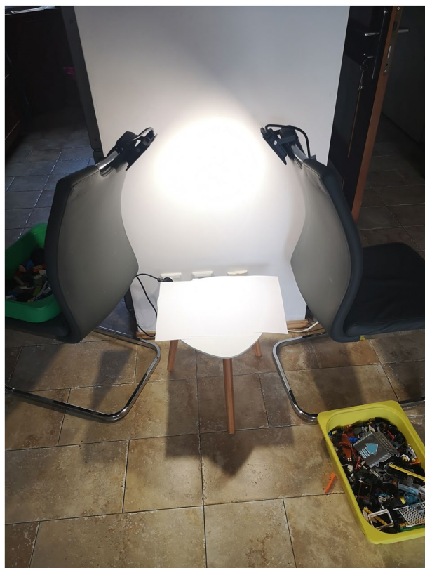
Fig. 2 Photo stand for taking images of LEGO bricks. Bricks of the same shape were spread on the white surface and the photos were taken using a hoovering handheld camera. The bricks' coordinates were automatically detected using a neural network.
