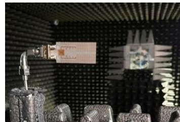
Figure 12. The radiation pattern measurement setup.
