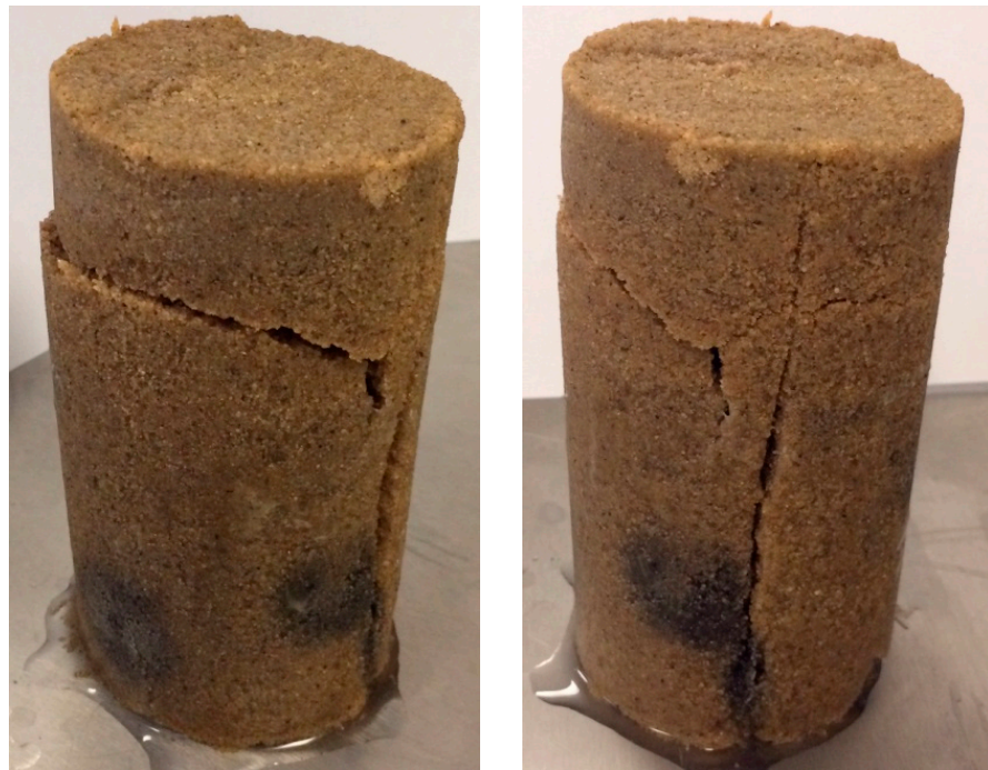
Figure 23. Specimen C2-23608 after 14 days of degradation in water.
