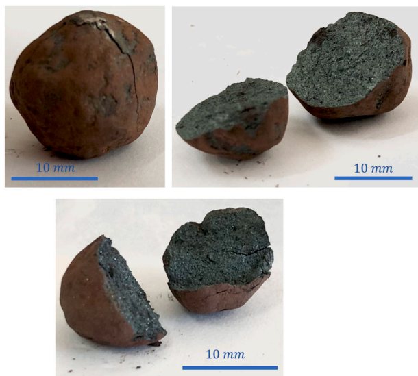
Fig. 11. Pellets aspect after the compression tests.
