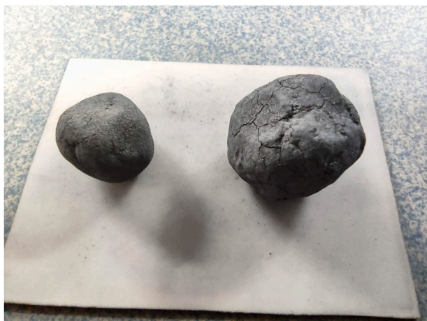
Fig. 13. Pellets reduced in hydrogen at 1000 °C.
