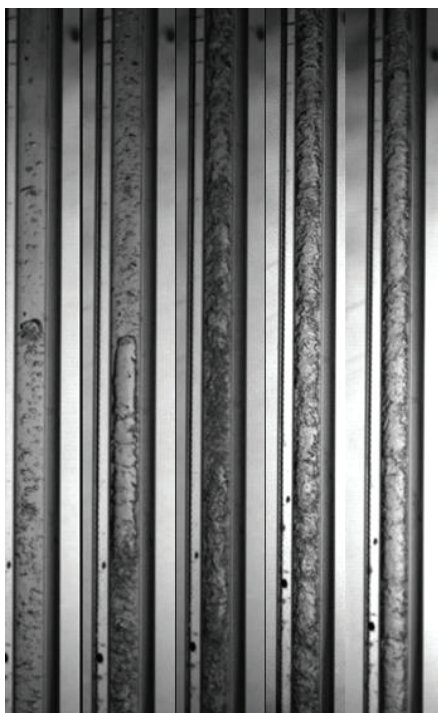
Figure 5. Flow Patterns Pr=0,6 G=355 \text{kg}/(\text{m}^2\cdot\text{s}) Quality respectively: 12%, 15,6%, 19,6%, 23,9%, 36,2%, 60,7%
