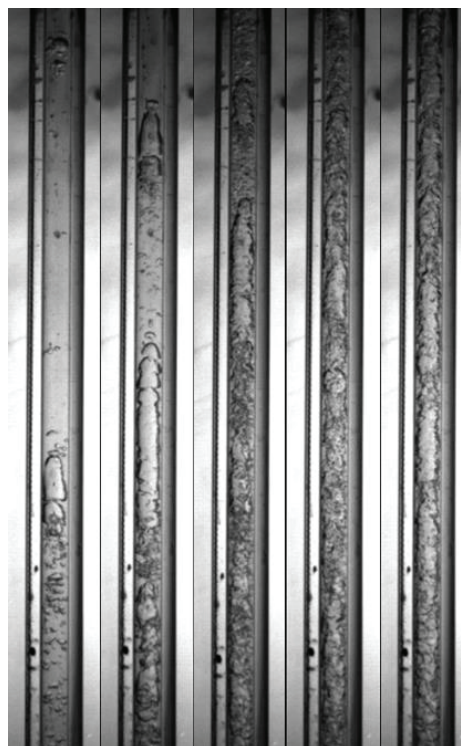
Figure 8. Flow Patterns Pr=0,6 G=180 \text{kg}/(\text{m}^2\cdot\text{s}) Quality respectively: 37,2%, 48,6%, 64,6%, 72,8%, 93%
