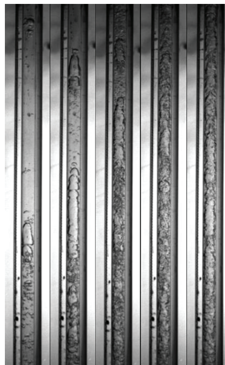
Figure 8. Flow Patterns Pr=0,6 G=180 \text{kg}/(\text{m}^2\cdot\text{s}) Quality respectively: 37,2%, 48,6%, 64,6%, 72,8%, 93%
