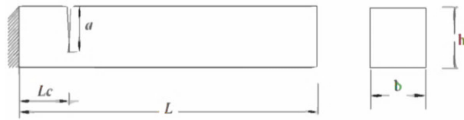
Figure 1. Model of a cantilever beam with crack.
