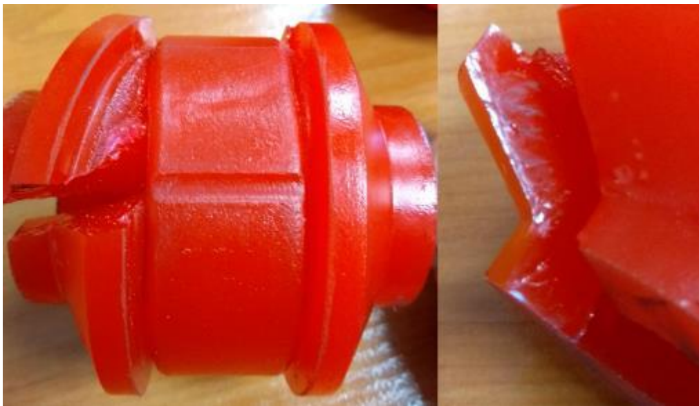
Figure 6 Damaged 80 ShA polyurethane sample (load level 20kN)
