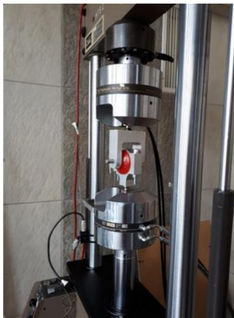
Figure 3 Specimen during fatigue test (80 ShA)
