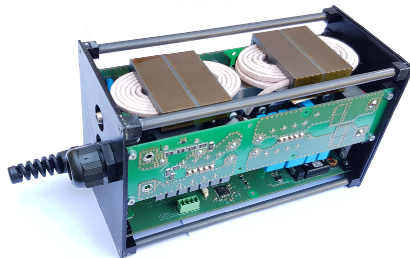
Figure 25. A photograph of the second prototype of the bidirectional isolated on-board charger.
