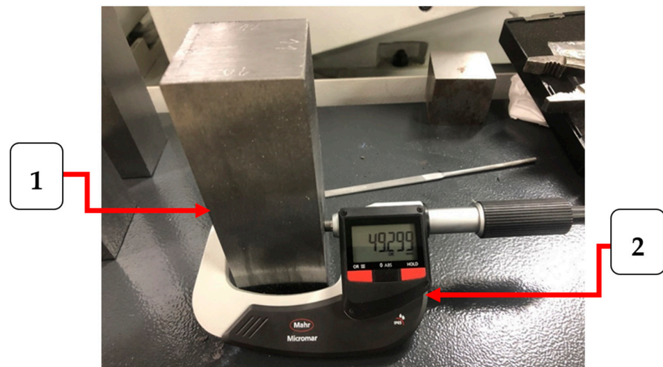
Figure 3. Measurement of the overall dimension of the ground workpiece: 1—measured workpiece and 2—digital micrometer.
